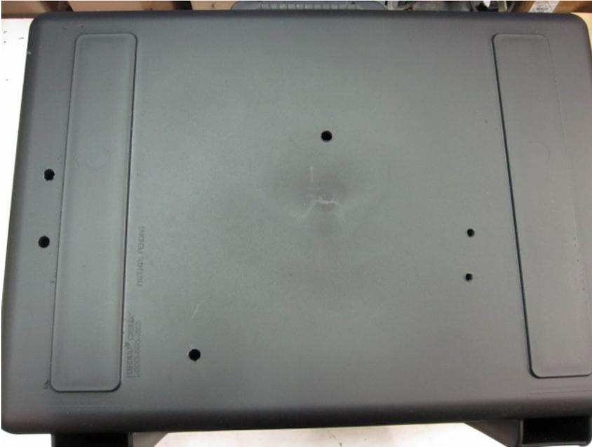
1) Assemble the parts onto the back of each case as shown in the photos below. Remove any plastic shavings from around the holes to allow a complete seal when the bolts are tightened (sealant is not necessary).
