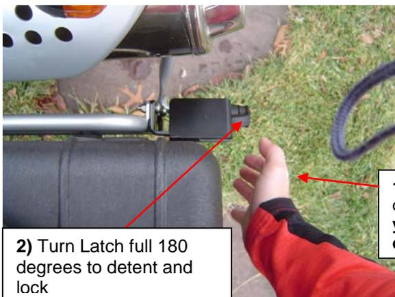
If the compression latch cannot be rotated fully clockwise to detent, check to ensure the front cleat is engage with the front rack tube and the latch is all the way forward on the latch plate. If the compression latch still cannot be rotated fully clockwise to detent, or it turns completely without a firm detent, adjust the jam nuts on each side of the red-tipped cam with 17mm wrench. Moving the jam nuts upward toward the latch bracket increases
