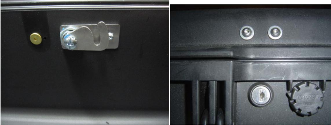
4) Install the strike plate to the lid. Place the two #10 washers on first, then fasten the strike plate with the #10-24 screws, sealing washers and nylock nuts.
