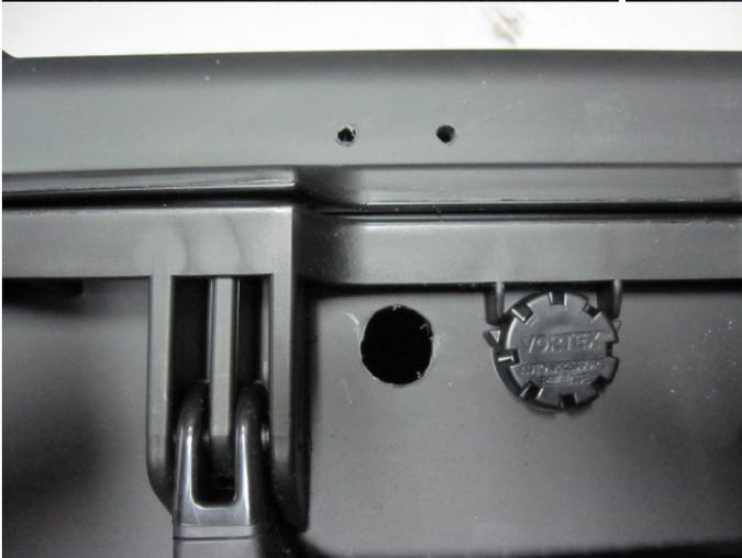
3) Assemble the lid lock into the big hole in the body and apply the double-d plate inside the case. Add some Loc-Tite to the threads on the lock barrel and tighten the big nut. Screw in the small #6 metal screw through the hole in the double-d plate and into the case (a small electric driver works well). Fasten the cam to the end of the lock barrel with the Phillips head screw (use LocTite on this screw).
